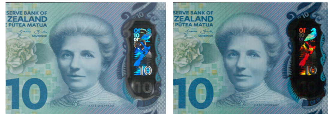
FIG. 4 - CHANGE IN APPEARANCE OF THE HOLOGRAPHIC THREAD UNDER TWO DIFFERENT ILLUMINATION CONDITIONS
