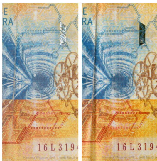
FIG. 6 - USE OF BALANCED (LEFT) AND ASYMMETRIC (RIGHT) ILLUMINATION TO DETECT CREASES AND CRUMPLING
