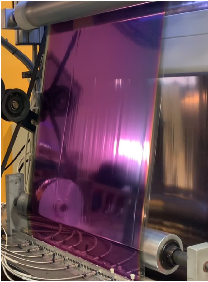
Figure 5: Complex thin film roll coater used to manufacture LumaChrome
